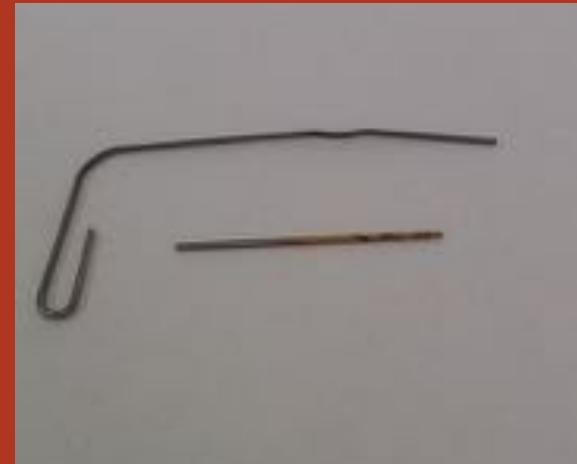
We take the clip and unfold one of its curves and select the Mini Drill Bits of the same diameter as the clip.
