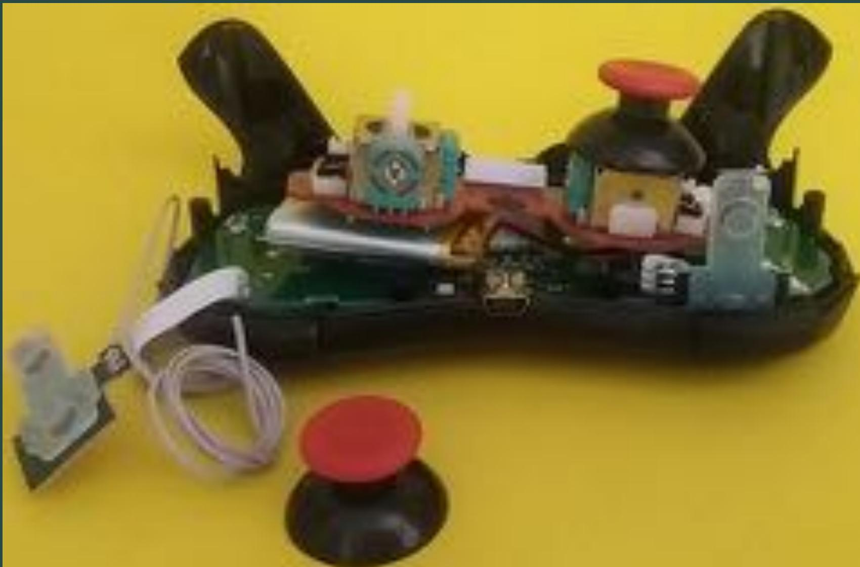
We will pull up gently, to separate the thumbstick from the joystick control
