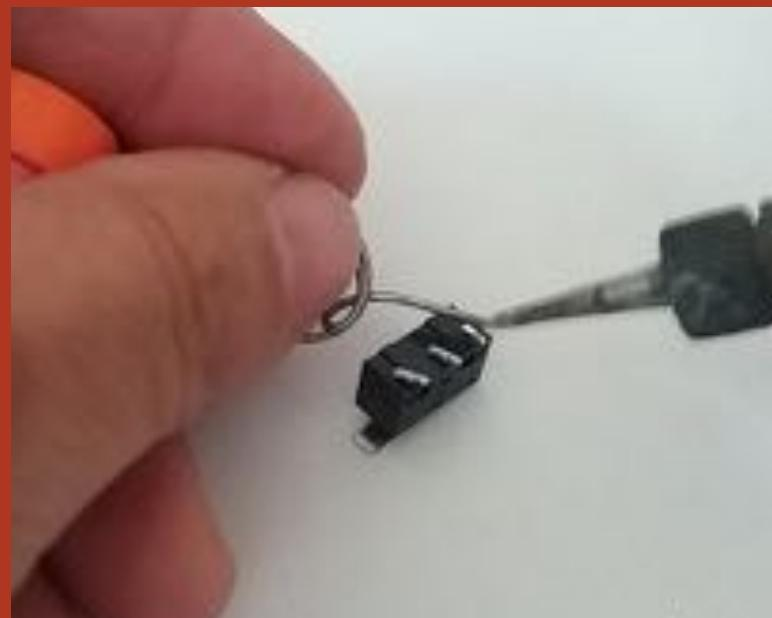
We bend the metal pins of the switch
