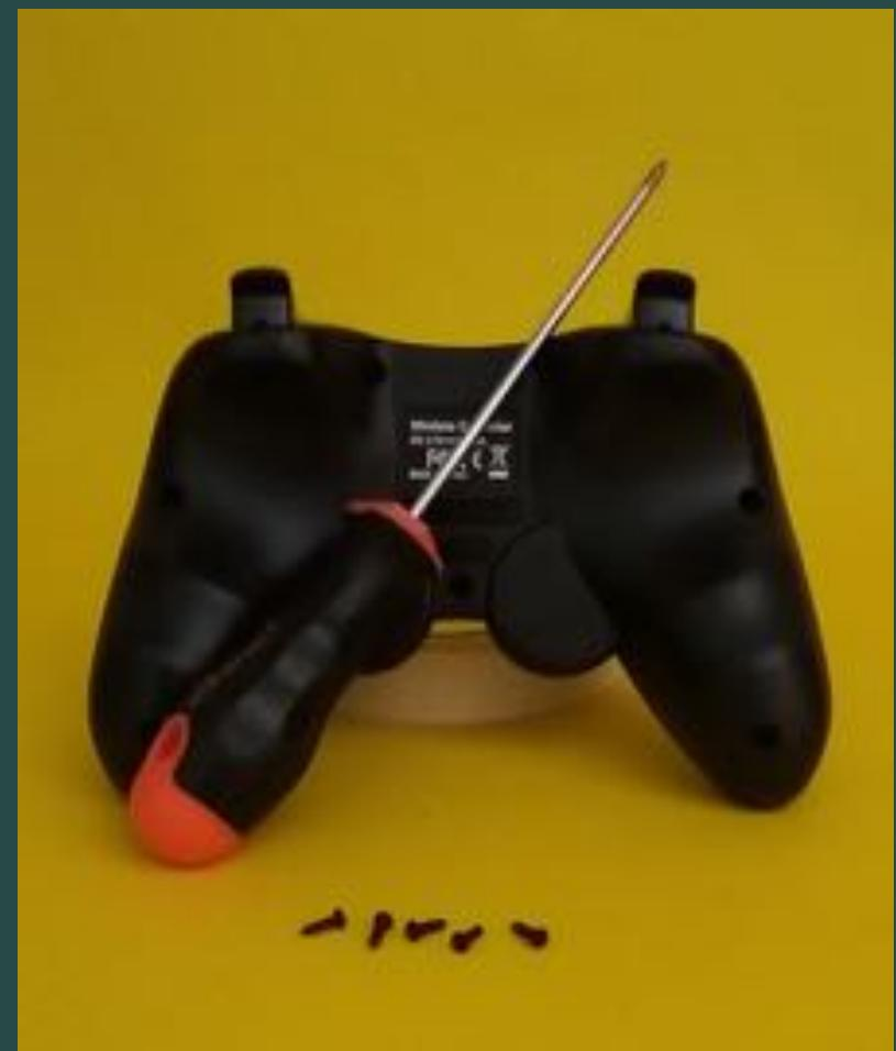
**With the screwdriver we remove all the screws,
