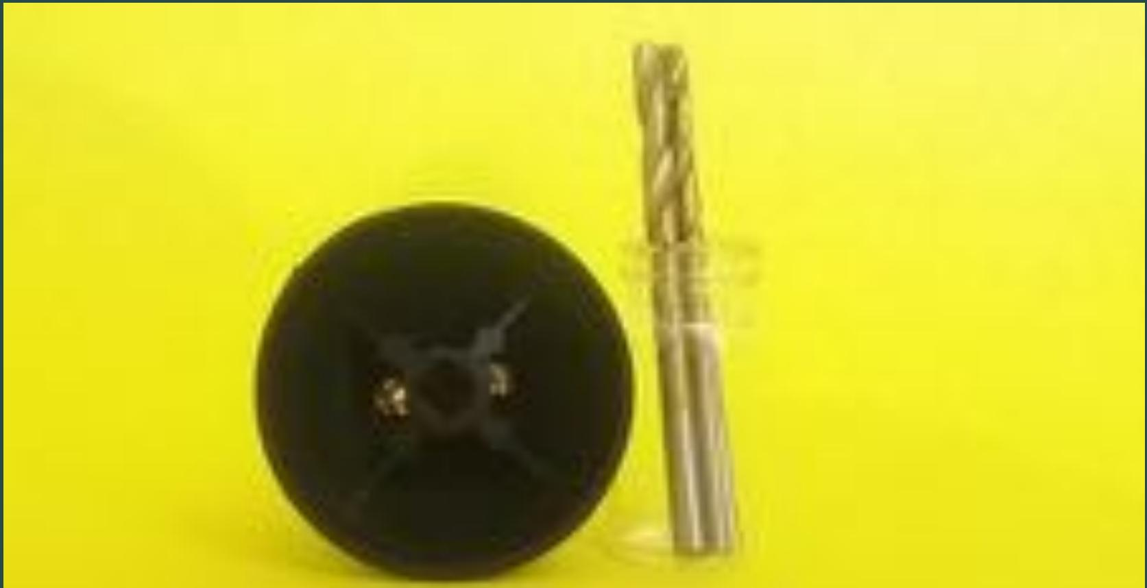
The diameter of the hole is equal to the size of the cable.
